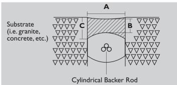
**Dimension A** - Joint Width **Dimension B** - Sealant Depth (over backer rod) **Dimension C** - Sealant Contact or Bond Surface
