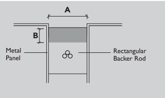
**Dimension A** - Joint Width **Dimension B** - Sealant Depth and Bond Surface
